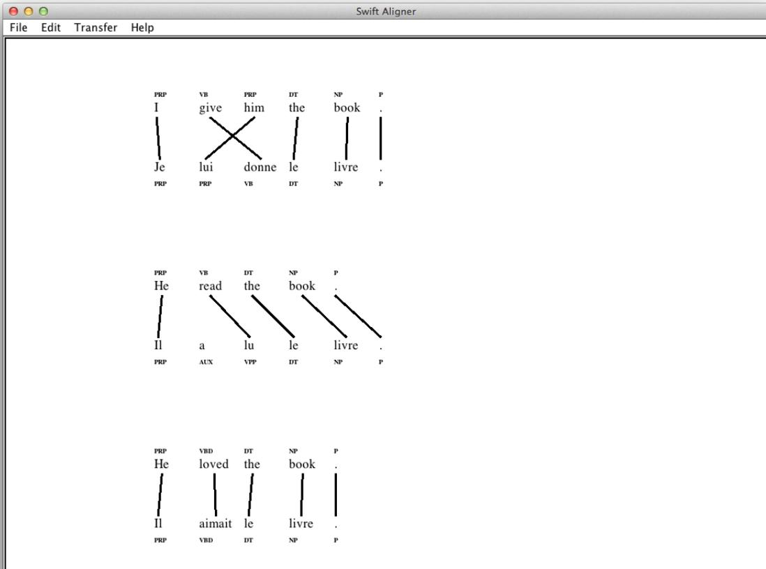
Figure 2: SWIFT aligner’s main GUI. Alignment between words in 3 different sentences is presented. POS labels are displayed for each word.
